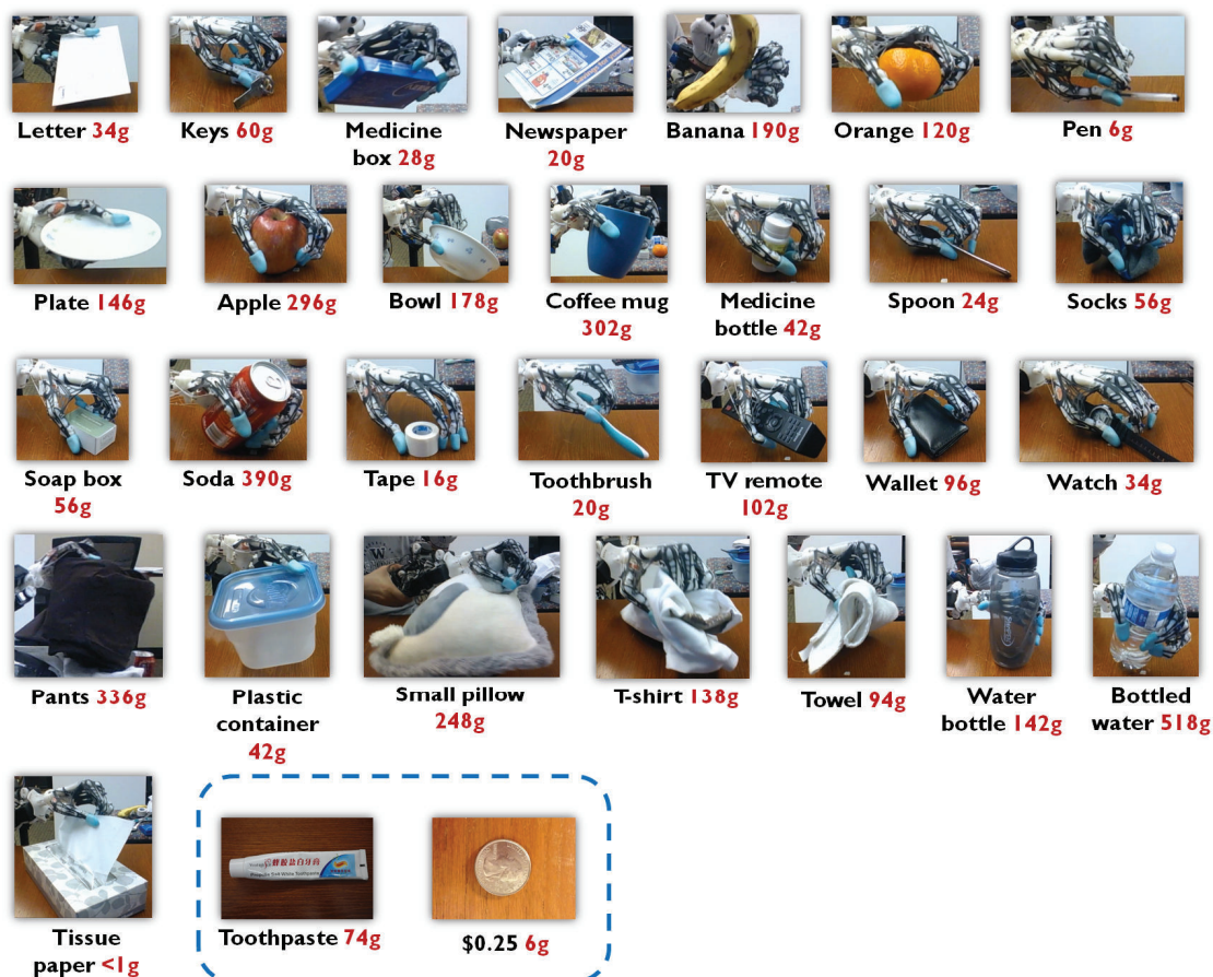
Figure 8.17: The list of objects used in the grasping tasks during tele-manipulation. Note: All the objects were initially placed on the table. The two objects enclosed in the dashed box are the ones that our robotic hand failed to grasp within four trials due to the flatness of the object, the slippery surface of the table, and limited vision at the grasping site.
