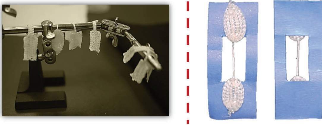
Figure 3.5: The preparation process of the tensile experiments. Left: Applying Epoxy on the two ends of the test samples. Right: In order to stabilize the flexible section, paper tapes were applied to both sides of the test examples.
