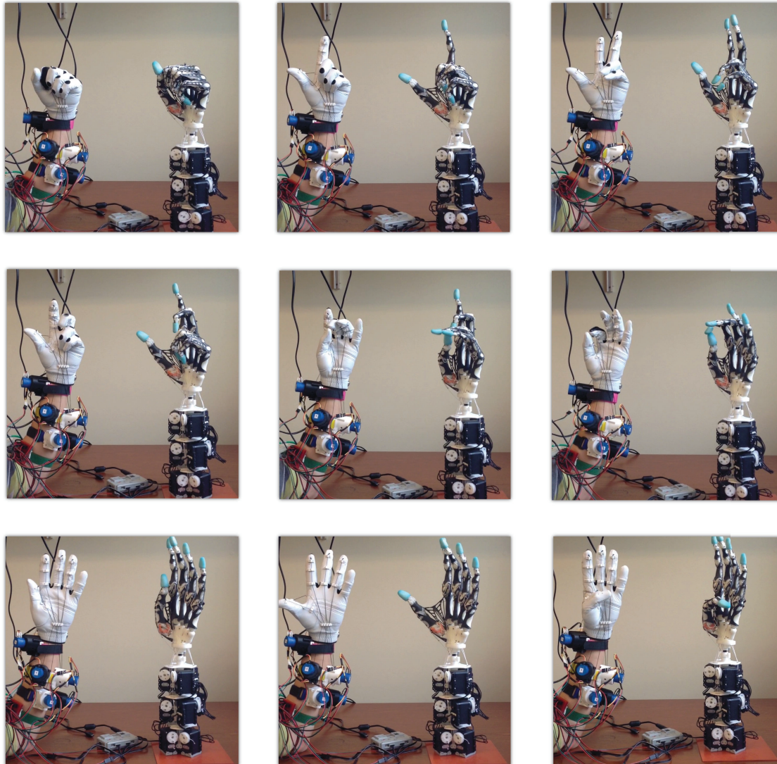
Figure 8.7: Snapshots showing the teleoperation process of our proposed anthropomorphic robotic hand. Top row: The index and middle fingers can move independently from the coupled ring and little fingers. Middle row: The precision grasp between the index/middle finger and the thumb. Bottom row: The abduction, adduction, and opposition motions of the thumb.
