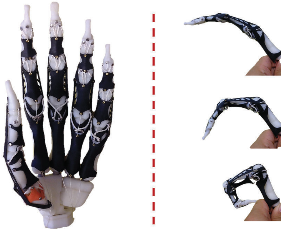
Figure 8.4: The elastic pulley system implemented on the palmar side of the biomimetic hand. Left: The flexor tendons of the robotic hand are running underneath the laser-cut, elastic tendon sheaths. Right: Snapshots of a separate finger showing the bulging process of the elastic pulleys during finger flexion.
