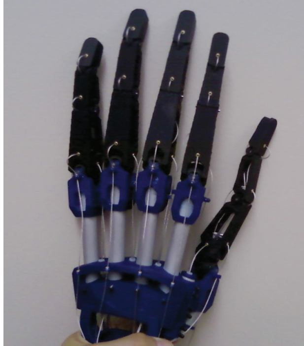
Figure 7.1: The 3D-printed 20-DOF anthropomorphic robotic hand.
