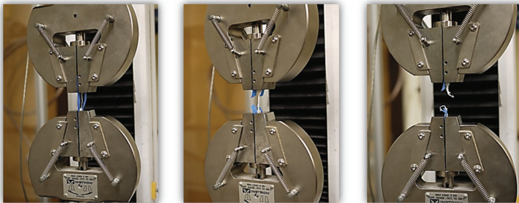
Figure 3.6: Example of the three stages of a typical tensile test. Left: The test sample was first loosely clamped at both ends. Middle: The two paper legs were cut before the pulling process started. Right: Pulling finished after the test sample reached its yield limit.
