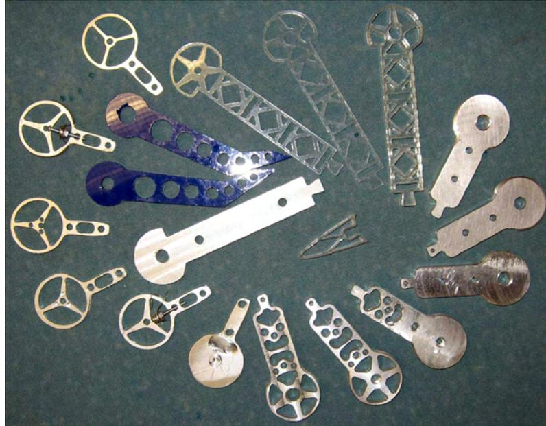
Figure 6.19: An example of one component's evolution from initial prototypes to final manufactured 6061 Aluminum component.
