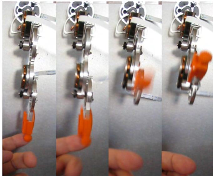
Figure 6.49: The passive dynamics of the robot are again displayed but this time along the first and second axes by a disturbance bringing about a large joint rotation in  $\theta_1$  and  $\theta_2$ .
