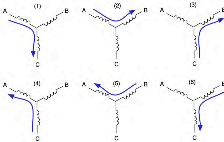
Figure 6.26: Block commutation sequence for a three-phase BLDC motor. Note the numerical sequence is the order, and that the third coil is left floating in each sequence.
