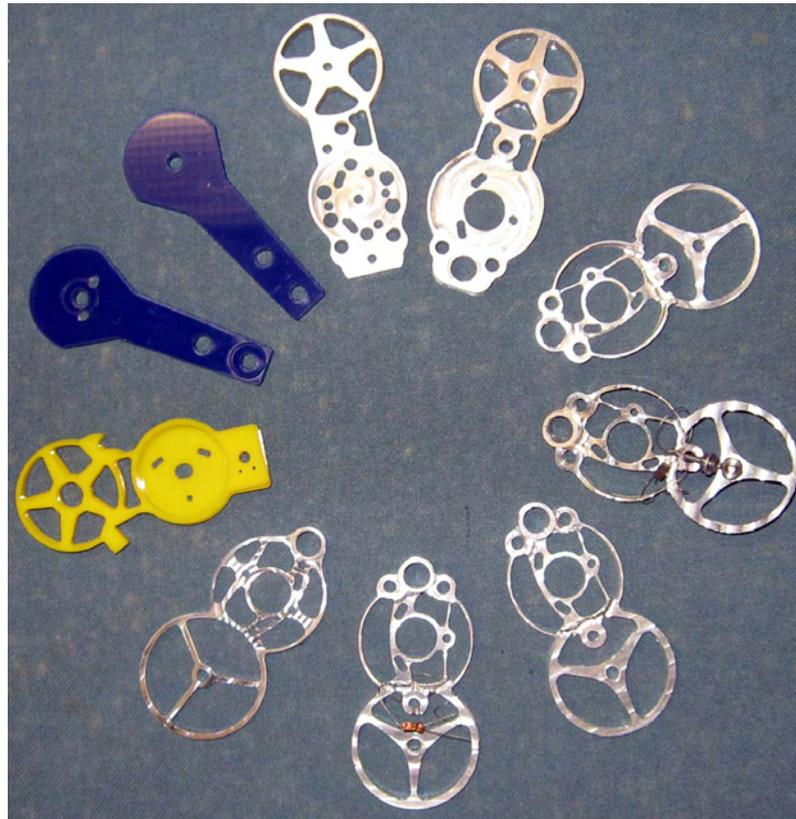
Figure 6.20: A second example of one component's evolution from initial prototypes to final manufactured 6061 Aluminum component.
