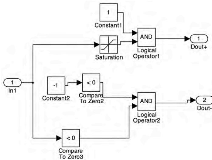
Figure 6.35: This depicts one of the circuit control logic blocks. Again, for computational efficiency bitwise logical comparisons are used.
