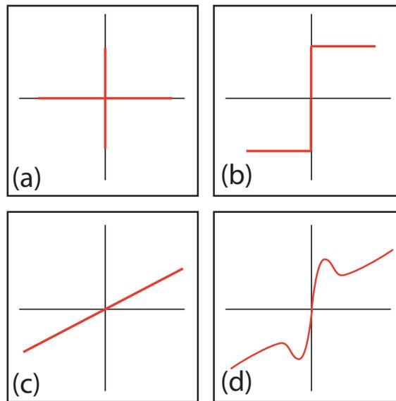
Figure 6.11: Models of friction. a, b, and c are, respectively, Stiction, Coulomb, and Viscous. d takes into account that friction is not discontinuous, and so captures the velocity-dependent friction components. This is referred to as Stribeck friction.
