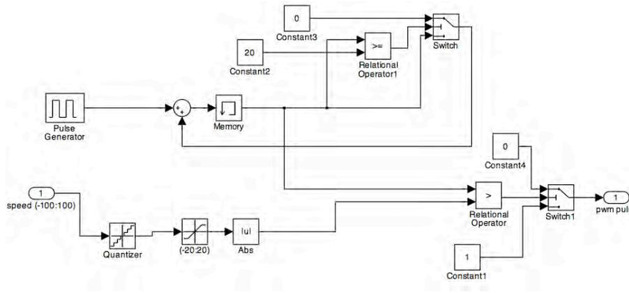
Figure 6.28: PWM generation scheme which works by repeating a cycle of pulses at a rate of 1kHz, with a number of pulses on versus off determining the PWM duty cycle (each pulse 20kHz frequency).
