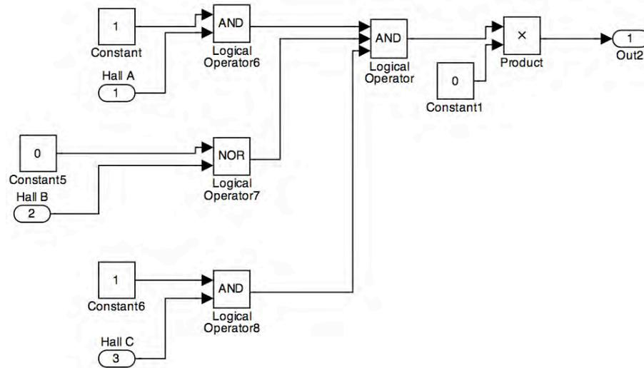
Figure 6.32: Detail of one of the six sector decoders. Only one will output a value per rotor position. Each one has a unique ID which is passed to the coil activation encoder.
