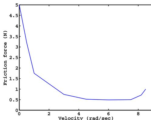
Figure 6.12: Friction of the motor characterized over frequency. The low frequency components are attributed to the Stribeck friction region, middle to Coulomb friction, and the high frequencies to the Viscous friction regimes. This plot, which represents an average over many trials, can be used to estimate parameters for the friction model.
