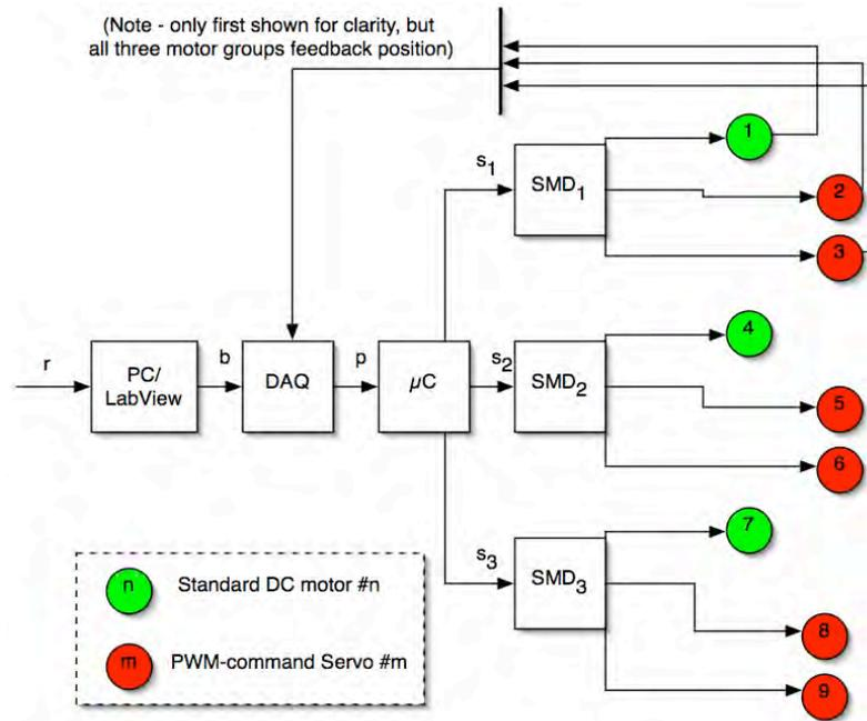
Figure 6.6: Block diagram for Tripedal Robot Prototype System (TRPS). The DAQ was a NI USB-6008 connected to provide analog outputs to a microprocessor which takes in the analog value and converts it to a motor torque command, which is then passed serially to the serial motor drivers (SMD). The motor drivers interface directly with DC motors and provide PWM pulses to two servos per driver. Position is measured with high accuracy low hysteresis potentiometers.
