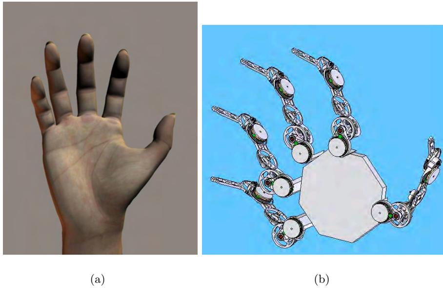
Figure 6.2: Depiction of (a) a human hand, and (b) a configuration of five ModBots arranged as fingers for an artificial hand.
