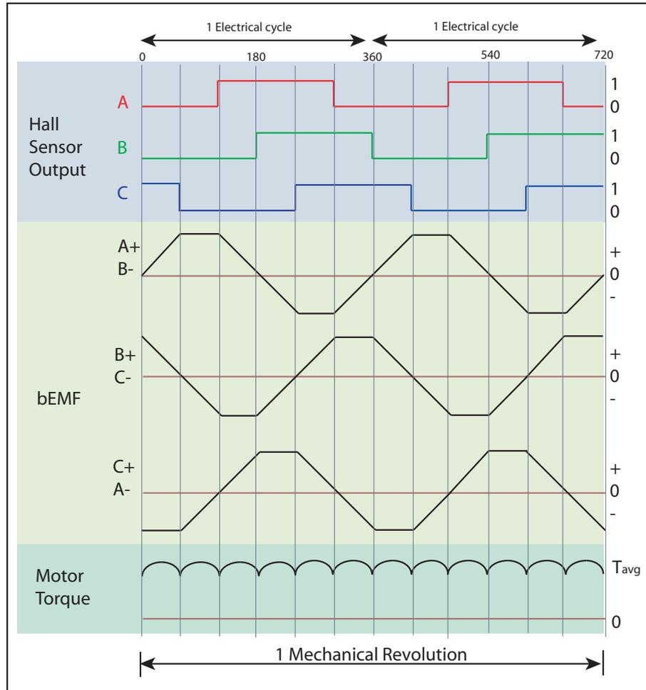
Figure 6.25: This denotes block commutation over one mechanical revolution for a typical two-phase BLDC motor with trapezoidal back-emf (adapted from AN885 technical note document from microchip.com). The torque ripple due to commutation is evident, and is undesirable for fine bio-mimetic control experiments.
