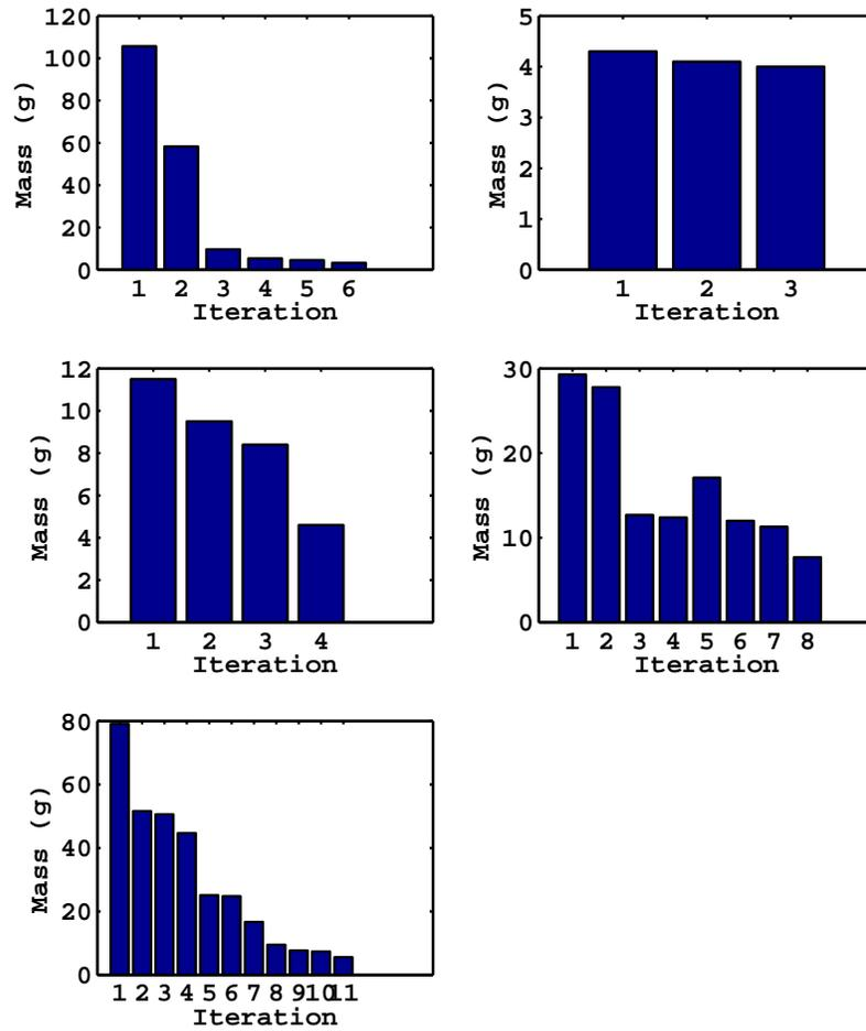
Figure 6.7: Bar plots showing the reduction in mass for each iteration of each component. Some components were developed in later versions of the robot, thus they had less reduction in mass (they were designed at a more evolved state of the robot).
