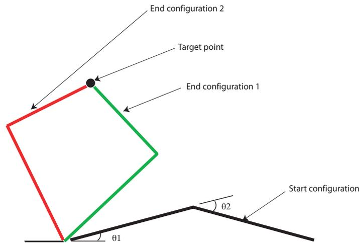
Figure 6.45: Given a target, there may be multiple configurations, and thus paths to attain that goal. Here we see two possible final configurations to reach a target point - green is one configuration, and red is another.
