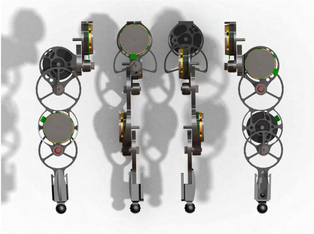
Figure 6.21: Left, top, bottom, and right projections of the modular robot leg design.
