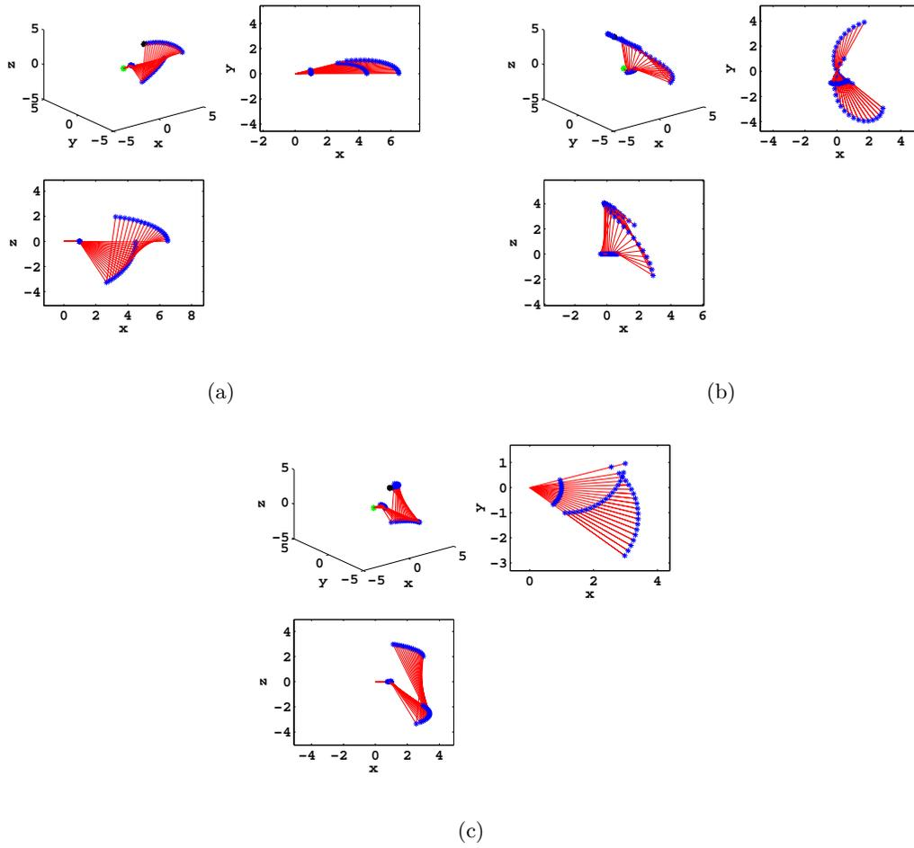
Figure 6.46: Demonstration of the Newton-Raphson algorithm computing the target joint angles, then the robot interpolates between start and target points to create a trajectory. Additional perspectives are provided for clarity.
