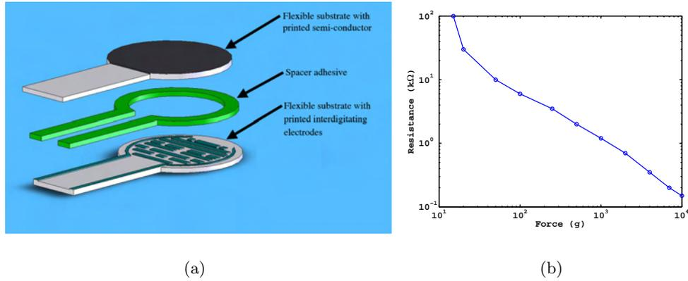
Figure 7.2: (a) Basic component structure of an FSR. (b) Average force-resistance relationship for a typical FSR.
