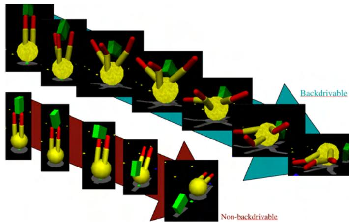
Figure 6.4: This depicts a block colliding with a multi-jointed system. One system is backdrivable, the other is not. The two systems (backdrivable and non-backdrivable) interact with the environment in fundamentally different and complex ways. It is difficult to force the non-backdrivable system to behave in the same way as the backdrivable system.
