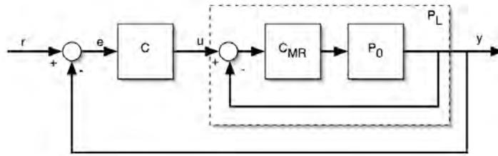
Figure 6.10: Model reference control design.
