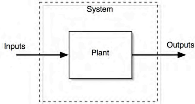
Figure 1.1: Relationship between inputs, outputs, the plant, and the overall system.
