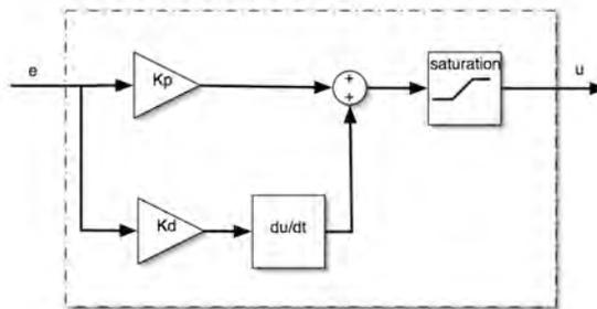
Figure 6.14: PD controller block diagram.
