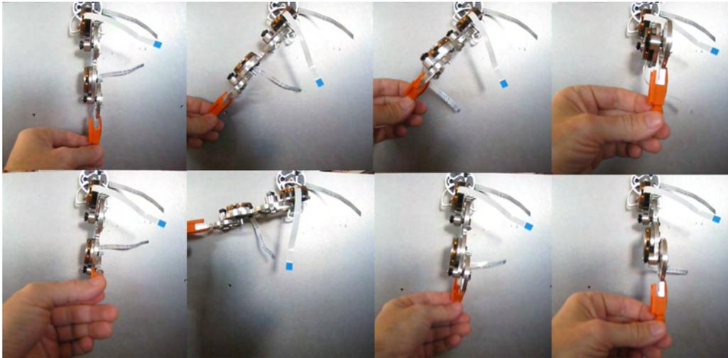
Figure 6.50: Here the robot is passively moved through a subspace of the workspace by a small external load (the human fingers pushing it gently).
