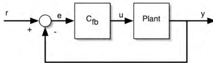
Figure 1.2: Relationship between inputs, outputs, the plant, and the overall system.
