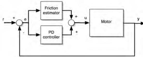
Figure 6.13: Compensation scheme block diagram.
