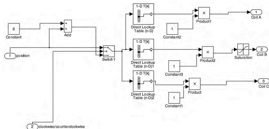
Figure 6.33: Lookup tables store the appropriate coil value per particular combinations of inputs.
