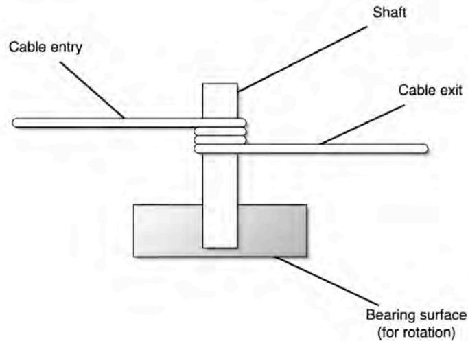
Figure 6.17: Basic cable wrap schematically
