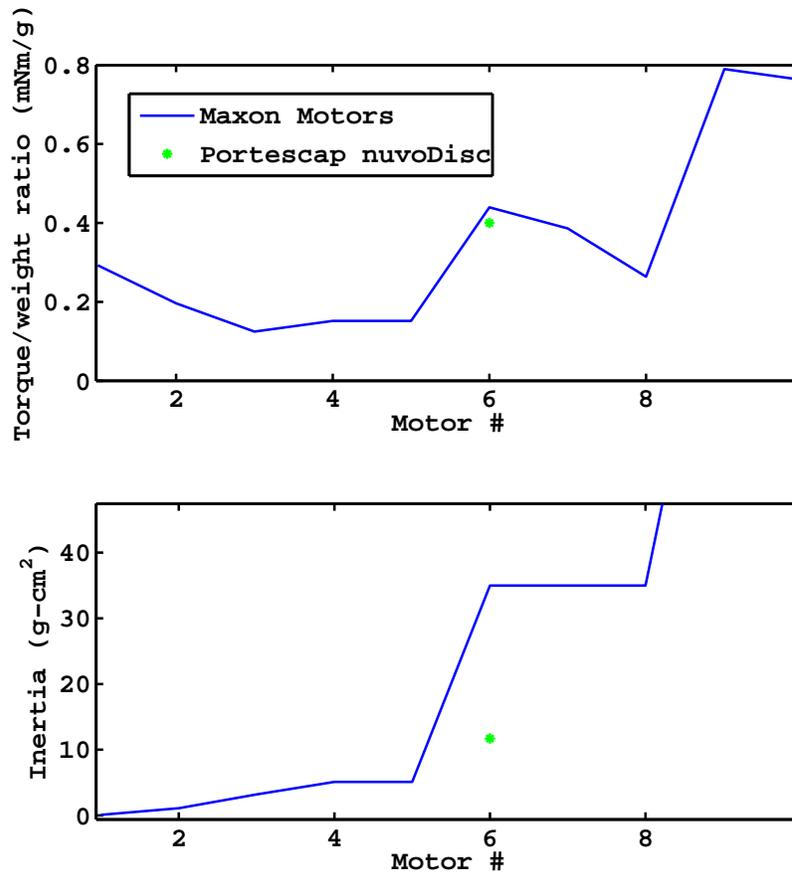
Figure 6.8: The motors were selected based on many properties, but the most key properties are mass, rotor inertia, and torque. Here it is clear that in terms of both torque-weight ratio and rotor inertia, the Portescap nuvoDisc brushless DC flat pancake motor is superior to the Maxon flat brushless DC motors. It has almost the same torque-weight ratio, but four times less inertia than the comparable Maxon motor.
