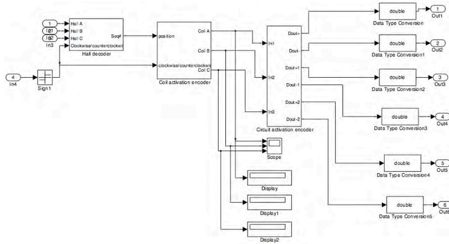
Figure 6.29: This depicts the overall Hall sensor decoding scheme. The three Hall sensors, corresponding to a 3-phase brushless motor's rotor electrical phase are used to decode a sector that the rotor is in. The coil activation encoder sends command to the circuit controller to activate a particular coil. The circuit activation encoder then flips appropriate logic bits to the FET transistors which create a positive, negative, or floating voltage in the appropriate coils.
