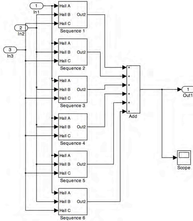
Figure 6.31: This is a detail of the Hall sensor decoding scheme. The appropriate value for each possible sector the rotor could be in is compared to the actual inputs as logical bit operations (which are very efficient computationally), and outputs the number of the sector
