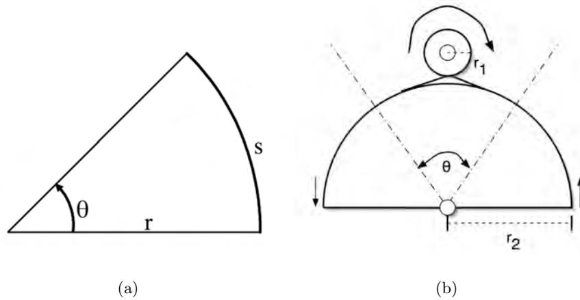
Figure 6.18: (a) Arc length, and (b) rotations of the small pinion shaft cause rotation of spur shaft, or linear motion along the cable direction.
