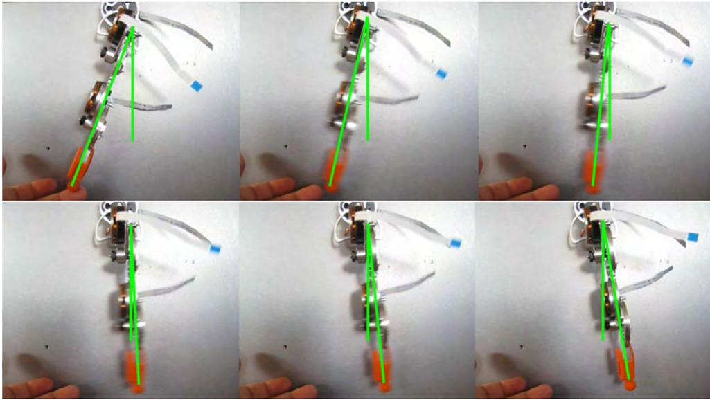
Figure 6.48: In this swing test the system can be seen to start from a raised angle in  $\theta_0$ , then when released it swings to an opposing angle. A robot without passive dynamics would not be able to achieve this in a simple way.
