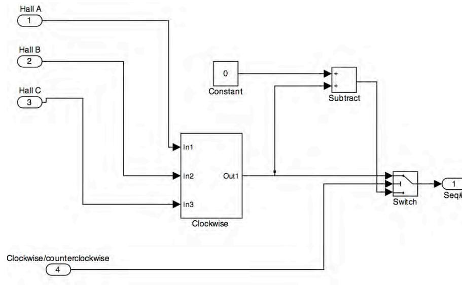
Figure 6.30: This figure depicts the Hall decoder, which has either a positive or negative direction component input.
