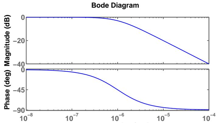
Figure 6.36: Frequency response of low pass filter for Hall sensors.
