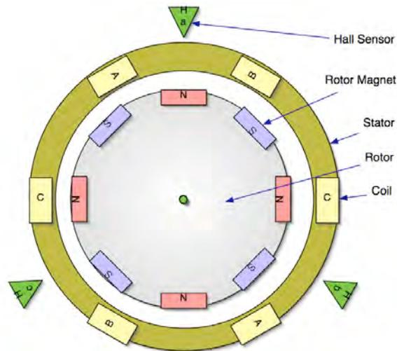
Figure 6.38: A simplified representation of a brushless DC motor with three phases and four pole pairs.
