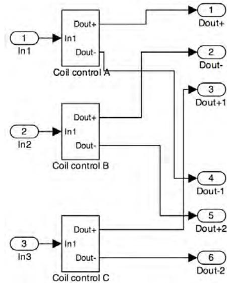
Figure 6.34: The circuit control logic determines, given a desired coil value for each coil, what pins to pull high or low in the triple h-bridge configuration circuitry.
