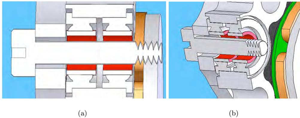
Figure 6.9: Section view of double ball bearing joint with nut removed for clarity. The use of precision high speed ABEC7 bearings, and all components pressed into place creates a very stiff (each bearing is rated to 250lbs. radial load) joint with an extremely low friction coefficient.
