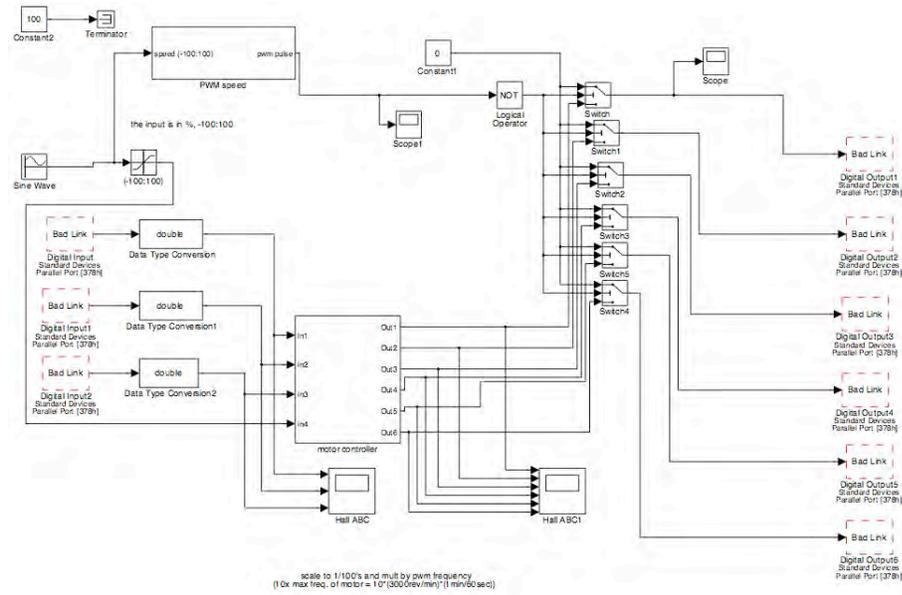
Figure 6.27: The overall view of the brushless motor block commutation model implemented in Matlab Simulink's Realtime Workshop.
