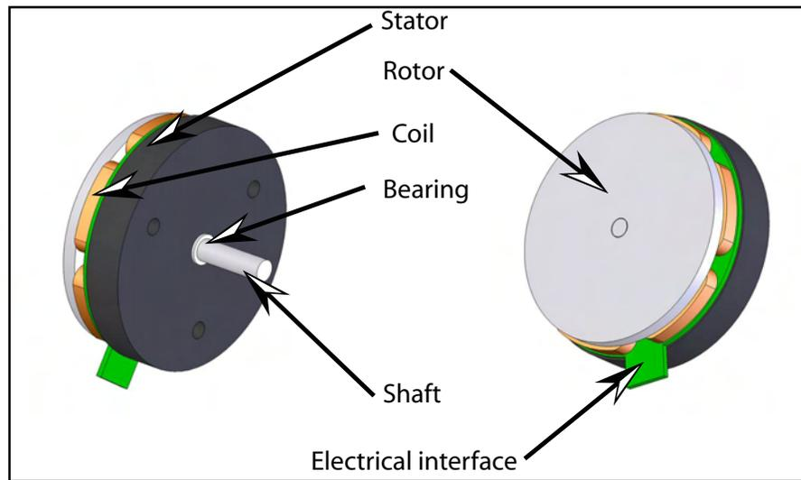
Figure 6.23: Basic components of a BLDC motor.
