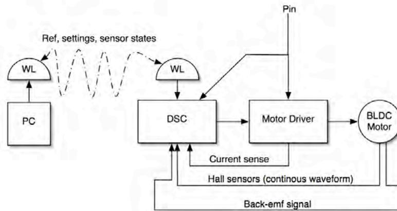
Figure 6.39: A block diagram representation of the motor control system, consisting of the PC providing, via bluetooth wireless connection, command reference, parameters, and receiving position and sensor data, the digital signal controller (DSC), motor driver circuitry, and BLDC motor.
