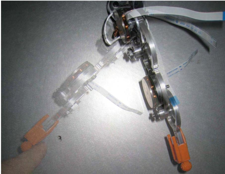
Figure 6.47: The robot's backdrivability allows the external world to affect the state of the robot; a must for manipulation tasks, and helpful for bio-mimetically realistic locomotion tasks.
