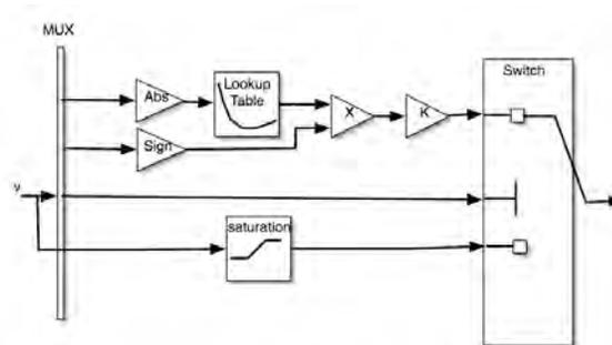
Figure 6.15: Friction estimator block diagram.
