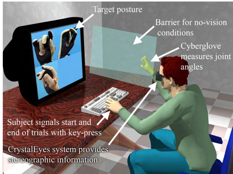
Figure 5.2: Image of experimental setup. Subject sits in front of a stereographic image system, with an optional barrier (depending on vision or no-vision condition) which obscures their hand. Postures are presented on the screen and the subject attempts to match those postures, with no time constraints.
