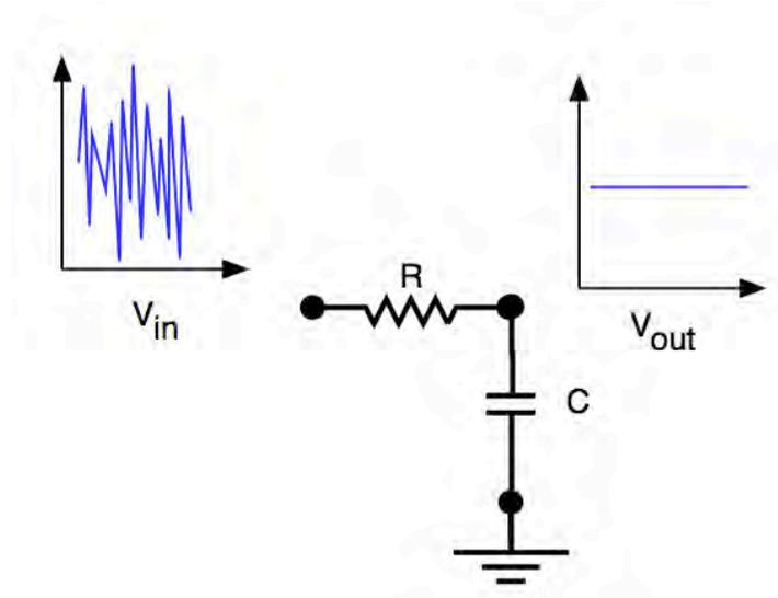
Figure 6.37: RC circuit, with  $f_c = \frac{1}{2\pi RC}$ , resistance in Ohms, and capacitance in Farads. The signal containing high frequency components enters the circuit, and leaves with high frequency components attenuated, leaving the lower frequency components intact.
