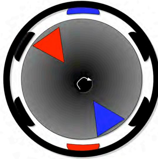
Figure 6.24: Simplified representation of a BLDC motor with torque created by applying a current through two opposing pairs of coils.
