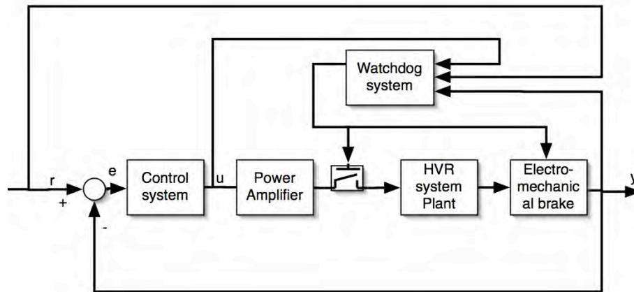
Figure 6.1: A safety method for human-robot interaction. A watchdog timer 'oversees' all important variables, and has the ability to cut power to the actuators and safely stop the system if values fall outside acceptable parameters.
