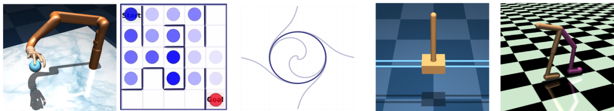
Figure 1.5: Some of the environments used for the control experiments. From the left, they are a robot arm picking up a spherical object, a discrete maze (red circle indicates the current agent’s position and the thickness of blue circles corresponds to the times the agent has visited those states), limit cycle dynamics, a cart pole, and a walker.
