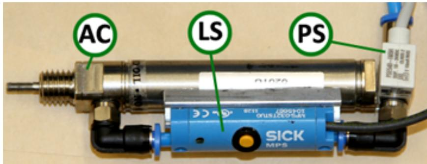
Figure 3.2: Cylinder unit [AC: Actuator, LS: Length Sensor, PS: Pressure Sensor]
