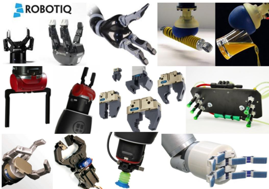
Figure 2.1: End effectors designs prevalent in the industry
