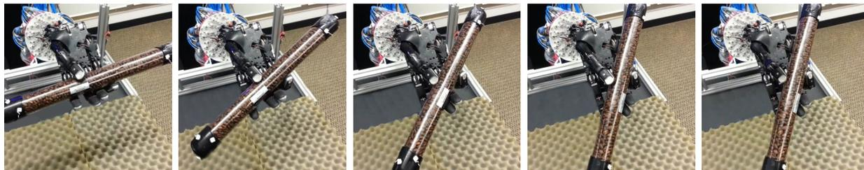
Figure 8.1: Learned hand manipulation behavior involving clockwise rotation of the object
