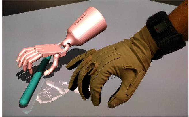
**(b)** Expert interacting with the simulation using Cyber glove system
