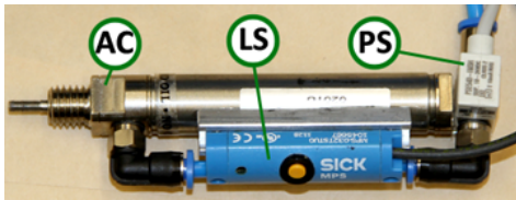
Fig. 2. Cylinder unit [AC: Actuator, LS: Length Sensor, PS: Pressure Sensor]
