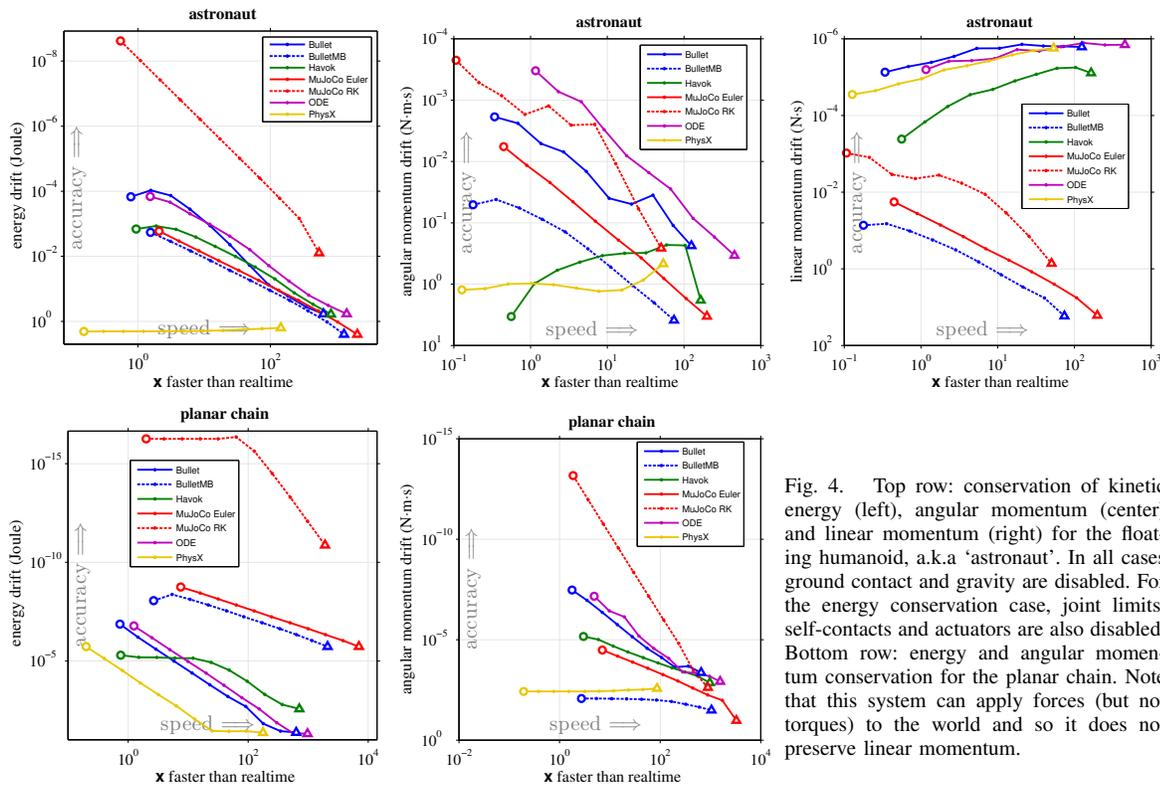
Fig. 4. Top row: conservation of kinetic energy (left), angular momentum (center) and linear momentum (right) for the floating humanoid, a.k.a ‘astronaut’. In all cases ground contact and gravity are disabled. For the energy conservation case, joint limits, self-contacts and actuators are also disabled. Bottom row: energy and angular momentum conservation for the planar chain. Note that this system can apply forces (but not torques) to the world and so it does not preserve linear momentum.
